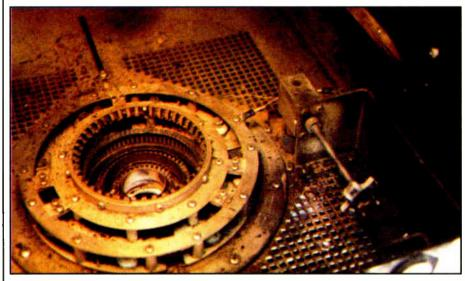
Fig. 4: Part of the final cavity of an RCA-BTF-20E1 transmitter damaged by fire.
