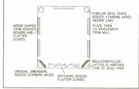
Fig. 1: Placement of Traps
