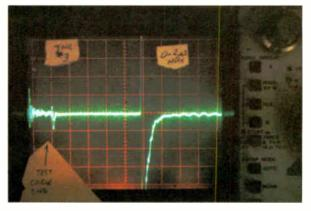
Figs. 1-3: An AM Station's Sampling Lines, Measured Using a Delta Electronics PRH-1 TDR
