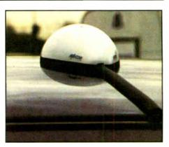
The N/A-COM roof-mounted antenna is one of two antennas Sirius featured on vehicles.
