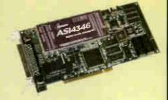
AudioScience's ASI4346 audio card features MP3 playback with on-board decompression. With it, MP3 audio files play quickly and smoothly. The card has four physical sereo outputs and one stereo input. It also includes a GPIO and an RS422 bitstream input, which supports direct input of a satellite receiver MPEG bitstream.
