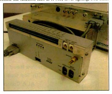
tery backup option in the event of a power failure to allow it to call specified phone numbers and inform the user of the failure.
