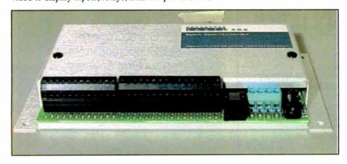
Connections are via screw terminals. A 12 VAC wall wart is provided with the system. Optional RM-2 or RM-3 rack panels each hold two units. The overall system is 7 x 1 x 4.15 inches and weighs 2 lbs. Retail prices start at \$469.
