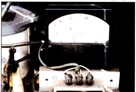
Fig. 2: Don't let connections get 'green' with corrosion, whether on a meter or on RF connections in the phasor or coupling unit.
