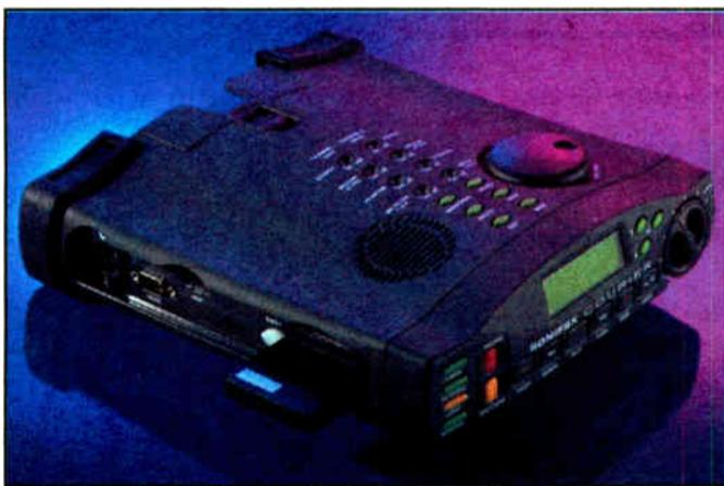
The Courier has been enhanced with a USB connection for downloads to a PC. The USB B connector supports USB 1.1, which has a theoretical data rate of 12 Mbps. Due to a Windows overhead, Courier USB data transfers have been carried out at 4 Mbps, which enables downloads to the PC of up to 60 times real-time speed (for ISDN based recordings at 64kbps).
