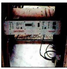
The FM 4000 consists of two Crown FM 2000s run through a combiner. Each FM 2000 has its own PA system and power supply.
