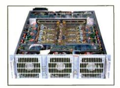
the TEX50LCD/S and TEX150LCD/S. Both come with adjustable power output, 0-50 W and 0-150 W respectively.
