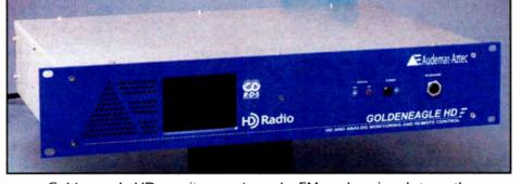
Goldeneagle HD monitors and graphs FM analog signal strength, pilot and RDS injection and HD Radio signal-to-noise ratio.
