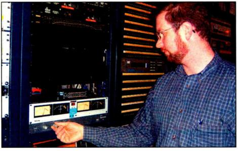
Evans likes the variable brightness adjustmen on th AVU-24's dual LED bargraph array. The unit sits above the McCurdy test set and the Symetrix amp that Evans is adjusting.
