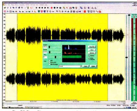
The EZ-Clean Filter removes pops, clicks, crackle and broadband noise in one operation, while visually showing what it is removing.
