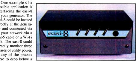
age limit, the easi-8 could start the generator. The easi-8 would then monitor the 3phase output voltage of the generator. Once up to voltage, the easi-8 would switch the generator on-line.
