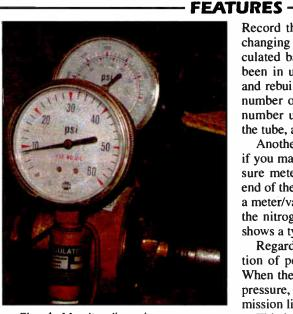
Fig. 4: Monitor line air pressure; it should never read zero.
