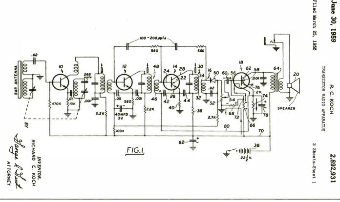
Patent application schematic for the transistor radio on which the Regency TR-1 is based.
