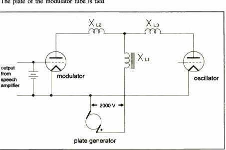
Heising modulation (adapted from Barton's 1925 thesis drawing).
