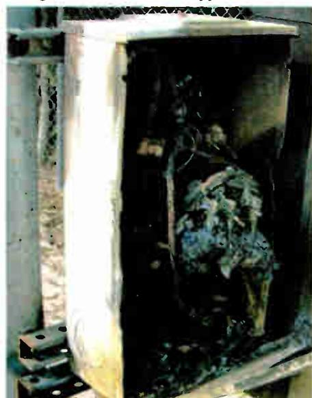
Fig. 2: Also not much left inside this 480 three-phase box.
