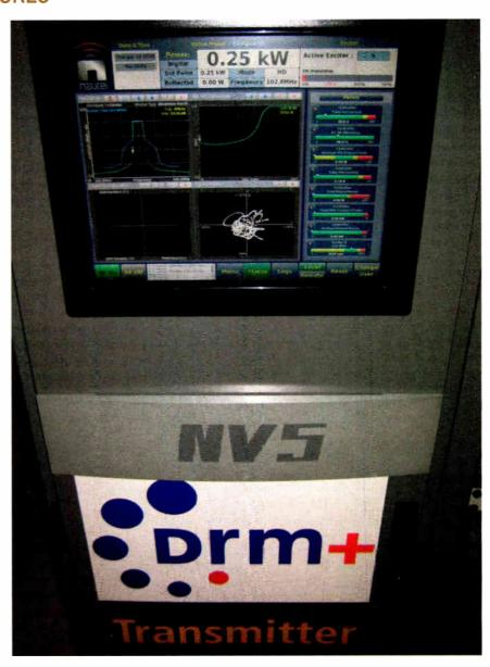
A Nautel NV5 DRM+ transmitter was used in the Hannover field trials.
