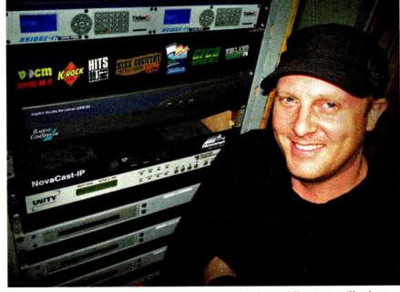
lic IP addresses at the studio and each of the transmitter sites. Using the Tieline multi-unicasting and AAC codec package at our St. John's studio allowed us to send high-quality AAC-LC audio at 128 kbps to these three transmitter sites in Labrador. We have been on air successfully to these sites for six months using Bridge-IT as our main source for stereo transmission, while the satellite is now our mono backup.
