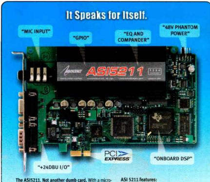
phone input, including a low noise pre-amp and 48V phantom power supply, on-board DSP, increased analog I/O level of +24dBu and a new GPIO that adds two opto-isolated inputs and two normally open relay outputs, the ASI5211 is one smart card. And considering it's priced the same as cards without all these features, it's one smart choice, too. For information, call us at +1-302-324-5333 or email us at salesasi@audioscience.com.
