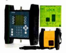
identify satellites by name, measure signal levels -70 to 10 dBm, plus display carrier-to-noise (C/N), signal quality, and Bit Error Rate. Confidently recognize the satellite a dish is aimed at, and peak the antenna to maximum performance.
