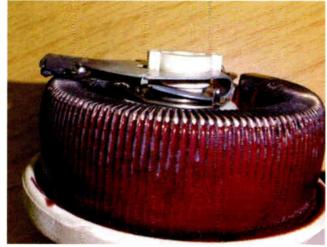
Fig. 4: The repaired rheostat with its solder blob contact.
