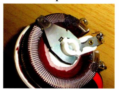
Fig. 2: A burned filament voltage rheostat.
