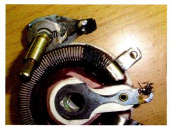
Fig. 3: Disassemble to repair the bad contact.
