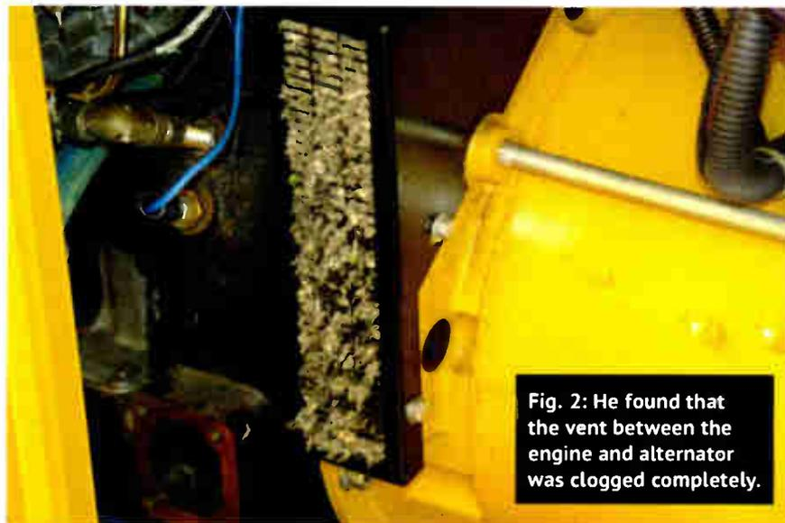
Fig. 2: He found that the vent between the engine and alternator was clogged completely.
