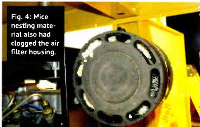
Fig. 4: Mice nesting material also had clogged the air filter housing.
