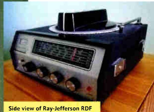
Side view of Ray-Jefferson RDF with large rotatable ferrite antenna for aiming at beacons.
