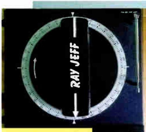
Top view showing 360 degree azimuth dial and rotatable ferrite antenna.
