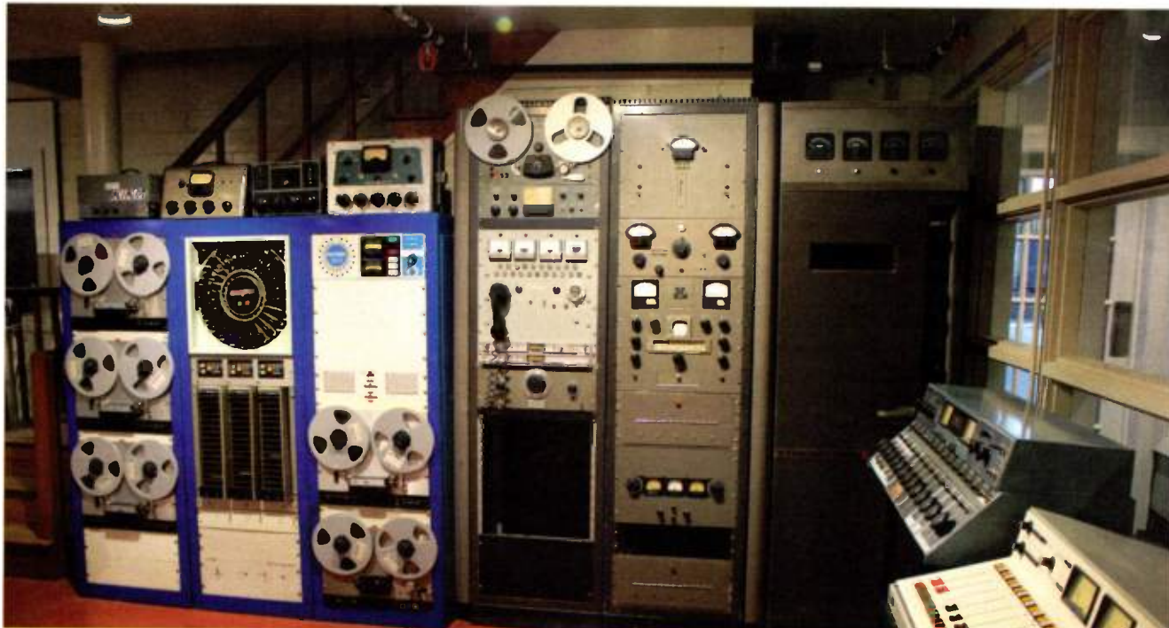
This seemingly ancient automation and playback equipment looks almost new. Starting on the left in the first rack group, on top of the Schafer 901 automation system are: a Marti remote unit, Raytheon, RCA and General Electric remotes mixers. The next group has, starting at the top, a Magnecord reel-to-reel recorder, a Schafer studio remote control, CBS Audiomax and Volumax processors and a Hewlett-Packard audio oscillator. The third group contains a variety of test equipment built by RCA and General Radio. The fourth group is an RCA BTA-1MX 1000 watt AM transmitter. On the far perpendicular right is a General Electric TV audio console and an Autogram console.
