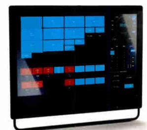
ruby's powerful visual interface is designed for fast-paced radio, with fingertip access to source, bus, and mix-minus assignments, as well as EQ and dynamics processing — freeing your talent to perform instead of searching for settings. You can even use ruby's GUI-building app to centralize control of studio software and peripherals. With intelligent AutoMix hands-free mixing and one-touch AutoGain mic calibration,
