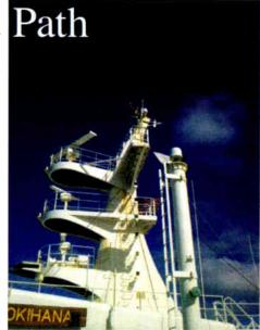
A view of the main mast of the MV Mokihana, showing navigational and communications antennas, including X Band and S Band RADAR, HF Radio, VHF radio, GPS and Standard-B, C, and Mini-M satellite domes. The author can be seen waving from its top.
