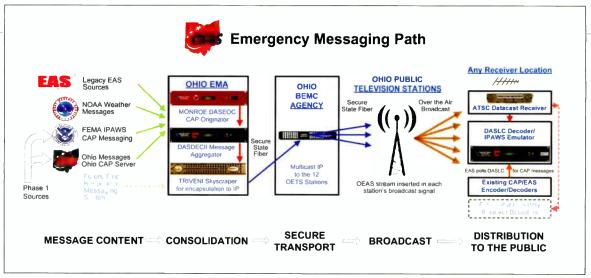
Ohio Digital EAS provides a simultaneous, redundant delivery path for current and proposed messaging systems. It's capable of delivering any digital signal format, as well as multiple formats.
