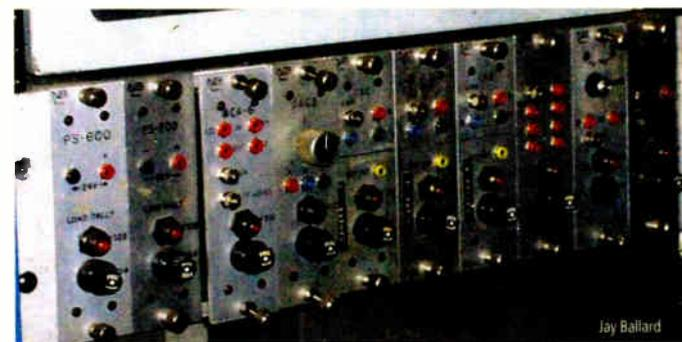
This surviving example illustrates the quality of workmanship turned out by NBC Burbank technicians. The frame contains DAs and a chroma keyer. Date of manufacture is roughly established by the network logo at the top left of each module. It was used between 1959 and the mid-'70s.
