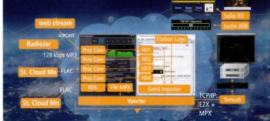
A graphic of the software-based airchain demonstration described in the article.
