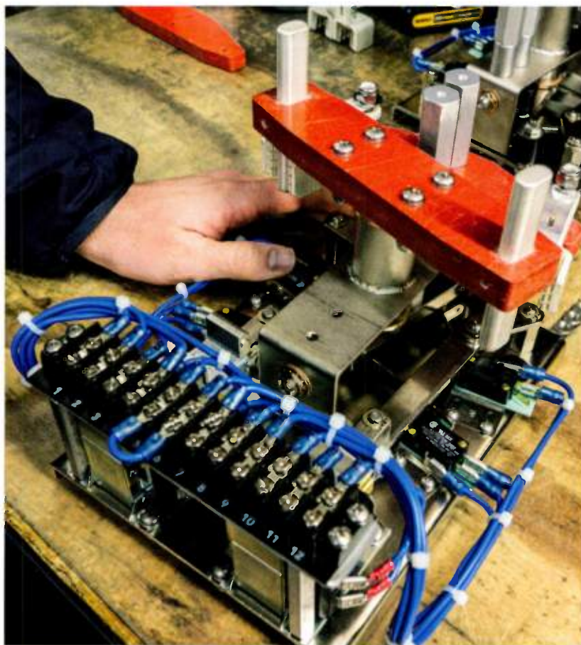
Above Fig. 1: RFC-40-20 RF contactor before final assembly.
