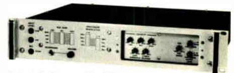
**RF Receiver/Generator**— A rugged, high output (2 watts) generator and correlation detector receiver virtually eliminate false nulls caused by interfering signals. The RG-3A operates from 0.5 to 1.65 MHz, and the expanded range of the RG-4 generates signals from 100 kHz to 30 MHz.
