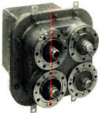
**Coaxial Transfer Switches**— These 1 3/8" and 3 3/8" motorized four port switches are designed to switch between antennas, transmitters, or dummy loads both quickly and efficiently. The switches can also be operated manually and are fully interlocked.
