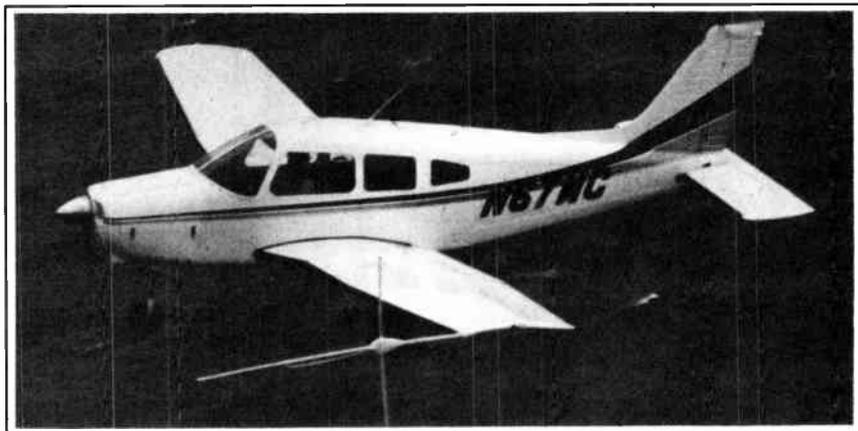
**A wing-mounted antenna helped Air System Technologies collect test data from the air.**
