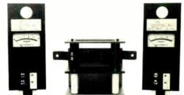
**Low Power RF Ammeters**— When every milliamp of current counts, depend on the accuracy of the TCA-Jr. This portable RF ammeter is designed to plug into either a Delta MJ-50 Meter Jack (pictured above), or a standard J-plug jack. Two current ranges are available: 0.2 to 1.0 Ampere, or 0.4 to 2.0 Amperes.
