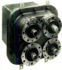
**Coaxial Transfer Switches** — These 1 7/8" and 3 1/8" motorized four port switches are designed to switch between antennas, transmitters, or dummy loads both quickly and efficiently. The switches can also be operated manually and are fully interlocked.
