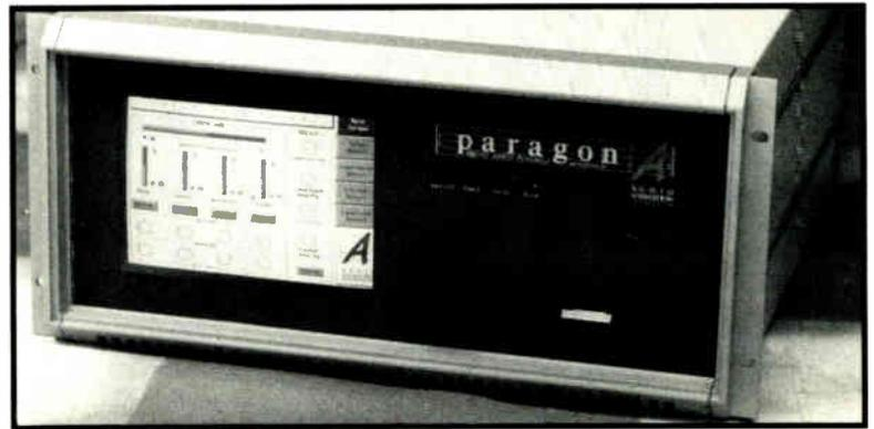
9" VGA touch-screen equipped video monitor; factory-loaded sound library; on-air A/B comparison; remote controllable. *User installable options* will include a Digital 10-band Graphic EQ, Stereo Generator and AES/EBU digital I/O.
