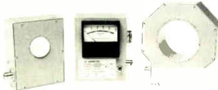
**RF Ammeters and Sampling Toroids** — Precision toroidal current transformers (TCT's) provide stable antenna monitor sampling while eliminating the problems associated with loops. TCT's also work well in supplying additional modulation monitor or test sample RF outputs. The transformer coupled ammeter (TCA) offers stable base or common point current readings, independent of modulation. The dual and single scale meters also provide remote DC outputs.
