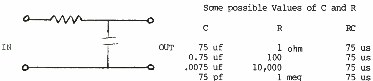
Figure 1. Simple Pre-emphasis Circuit
