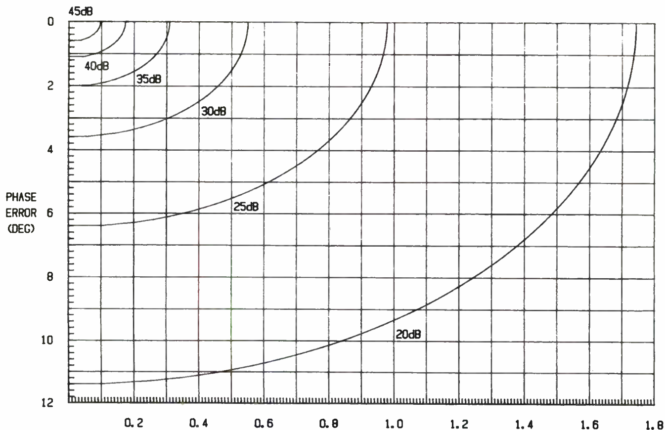
Figure 6. Separation vs. Differential Amplitude and Phase
