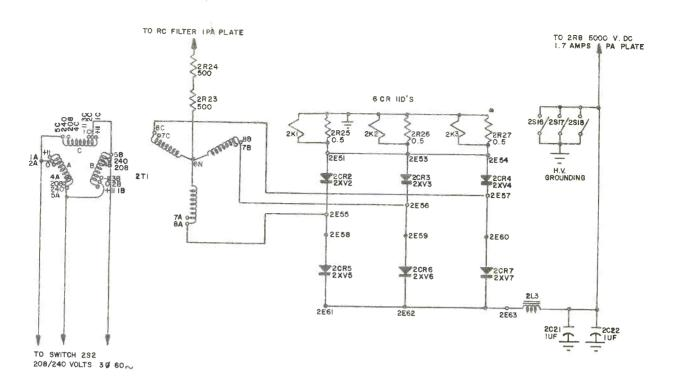
Figure 3. Schematic Diagram of the High Voltage Silicon Rectifier Circuit.
