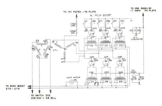
Figure 1. Schematic Diagram of Original BTF-5B High Voltage Power Supply.
