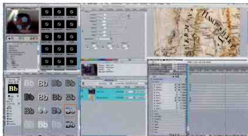
The Boris Red 3GL user interface has quick controls for many functions at the bottom of each window, as well as full menu access for all functions.
