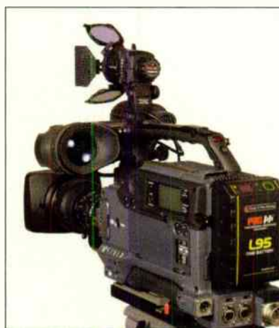
PAG batteries attach to a regular three-prong mount, eliminating retrofits.
