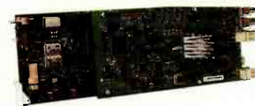
The Evertz 710XUDC-AES4 HD up/down/cross converter
