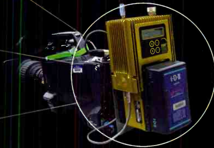
HDTV Camera-Mounted Transmitter with integrated camera-control
