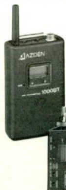
Bodypack transmitter (1000BT) with reduced current-drain for improved battery life, is available with Azden EX-503H, Sony ECM-44H.
