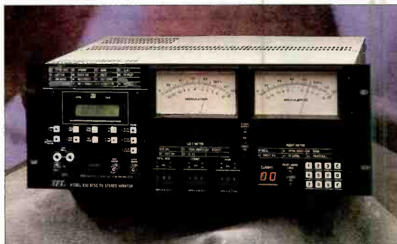
This popular monitor from TFT Inc. was used to monitor BTSC stereo when broadcasters began transmitting stereo audio in the 1980's.
