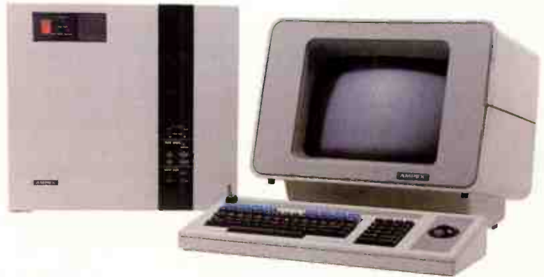
Introduced in 1985, the Ampex ESS-5G Graphic Composition and Storage System boasted a whopping (for its time) capacity of 160 MB and even had a crude asset management system via an "on-line cataloging function."
