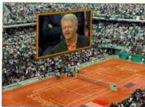
Orad's Cyberset technology allows broadcasters to combine up to four different video sources; the Jumbotron image of former President Bill Clinton is a different feed received from another camera inserted in realtime to the main feed.
