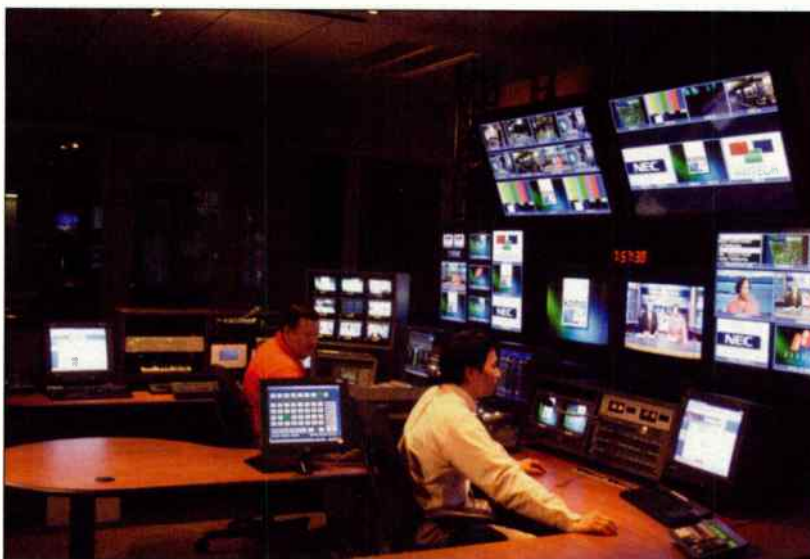
When KOMO-TV, the ABC affiliate in Seattle, upgraded its control room to handle HD, the traditional monitor wall was replaced with a plasma display.
