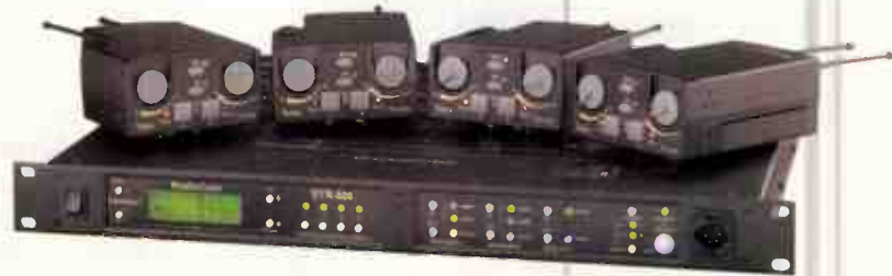
The Telex BTR-800 multichannel system uses UHF frequencies and diversity reception to improve performance.
