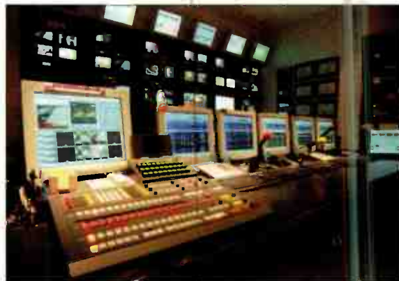
Emmis uses Florical automation to control five stations in a centralcasting system.
