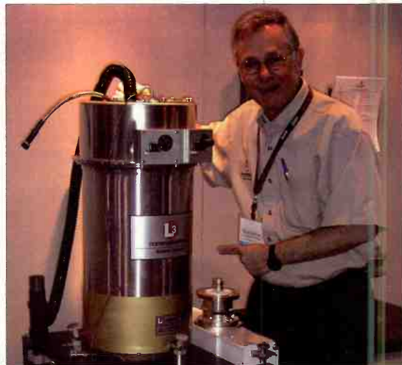
Buzz Miklos of L-3 poses with the company's Constant Efficiency Amplifier (CEA) MSDC IOT, an oil-cooled tube that promises efficiency as high as 60 percent.
