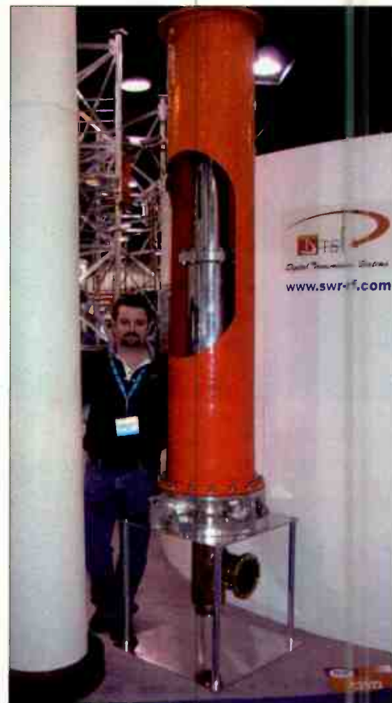
David Edmiston, Jr., of SWR poses with the company's dual-feed stacked-aperture UHF/VHF antenna assembly.
