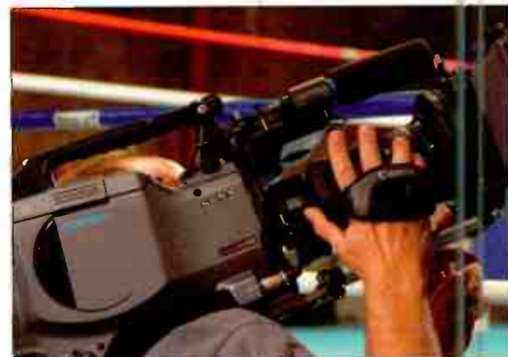
Sony's XDCAM system uses a blue-violet laser to record more than 23 GB on an optical disk.
