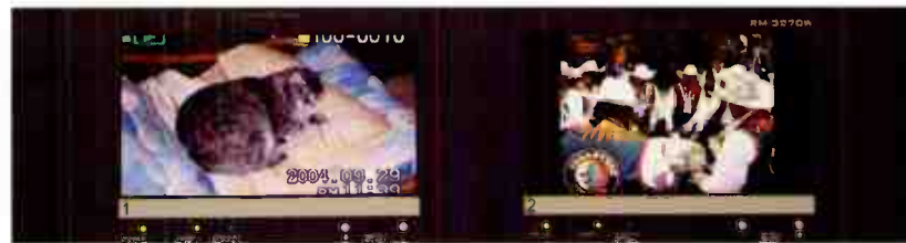
The Panoramadv RM-3270W has two seven-inch 16:9 LCD monitors, each with two analog inputs. An SDI input adapter can be added to either or both monitors.
