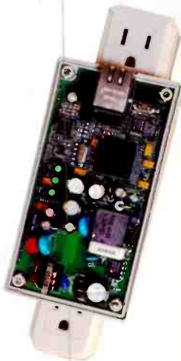
Pictured at right is Valencia, Spain's Design of Systems on Silicon (DS2) DSS9010 chip, in a board that plugs into a regular wall socket and moves A/V content on a home network at 200 Mbps.
