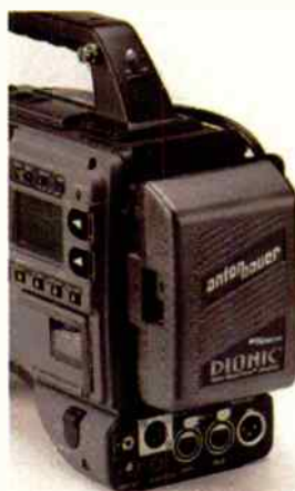
The Anton/Bauer Dionic 90 is a 90 W-h Li-Ion battery.
