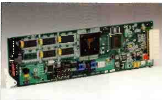
The Cobalt Digital 5821-D is an HD downconverter with aspect-ratio conversion and NTSC field lock.
