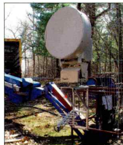
This 18 GHz DS-3 link provided by Total RF was used at the 11- and 18-mile points for the Boston Marathon
