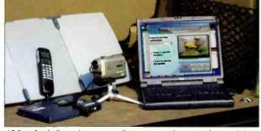
AP Snapfeed allows the user to edit a story on a laptop and transmit it to the newsroom over any type of wireless connection.
