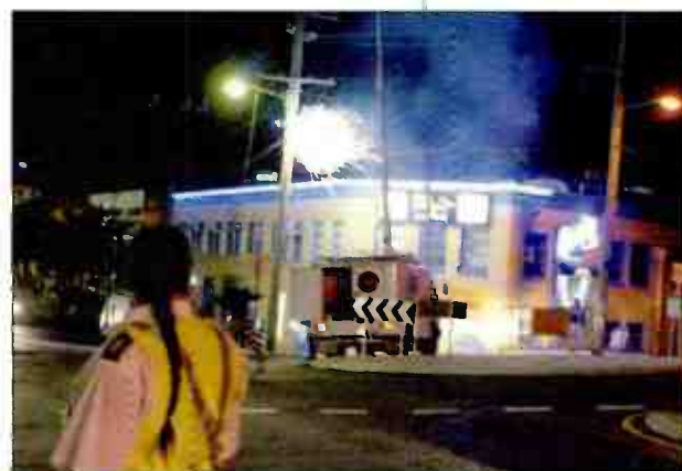
This ENG truck mishap in Australia illustrates the dangerous results when masts hit power lines.
