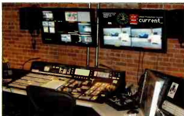
The Current facility includes a Ross Synergy switcher and signal processing gear from Miranda.
