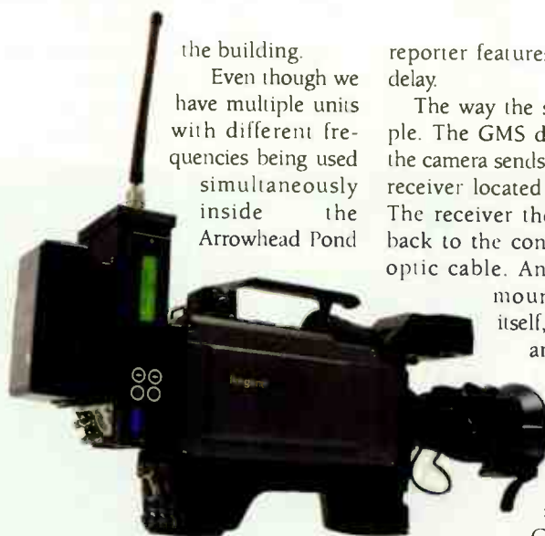
The Global Microwave Systems digital transmitter in place and ready for action
