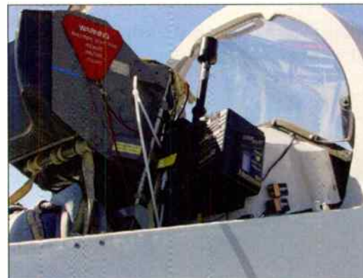
An RF Central transmitter on a MiG ejection seat
