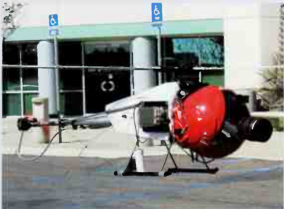
Flying-Cam UAV with GMS HD Messenger Link
