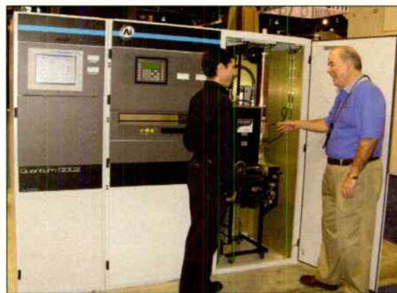
Dan Traynor of Acrodyne (R) points out the e2v MSDC IOT in an Ai Quantum transmitter to Alan Wheelhouse of e2v.
