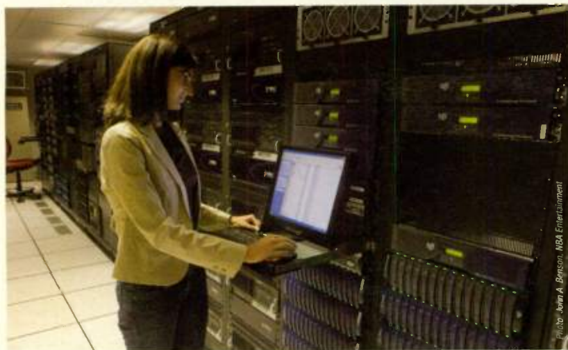
SGI InfiniteStorage SAN with CXFS shared filesystem provides real-time storage for 17 online Pinnacle Liquid Blue NLEs and storage for Virage low-res browse and retrieval.
