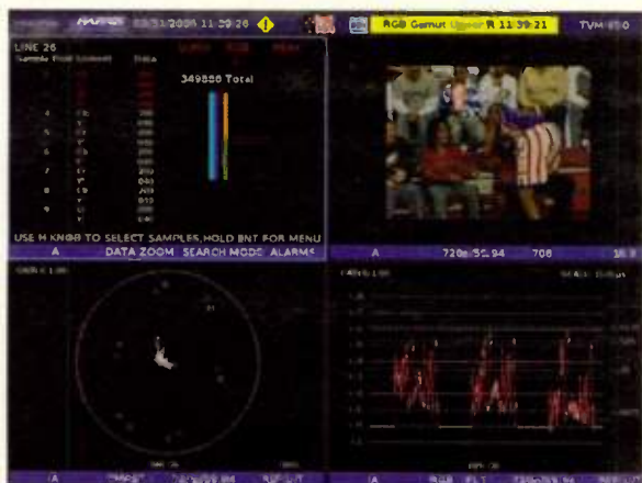
Data Analyzer display, with gamut errors highlighted (in red)
