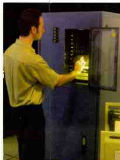
The SAMMA robot can hold from 40 to 60 cassettes at a time from the U-matic, Beta and/or VHS families.
