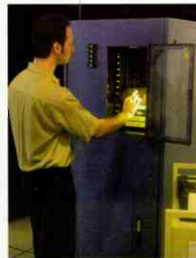
The SAMMA robot can hold from 40 to 60 cassettes at a time from the U-matic, Beta and/or VHS families.
