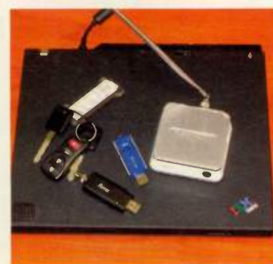
The FusionHDTV 5 USB Gold (the square box), the black Artec T14A and, for comparison, car keys and a USB flash drive.
