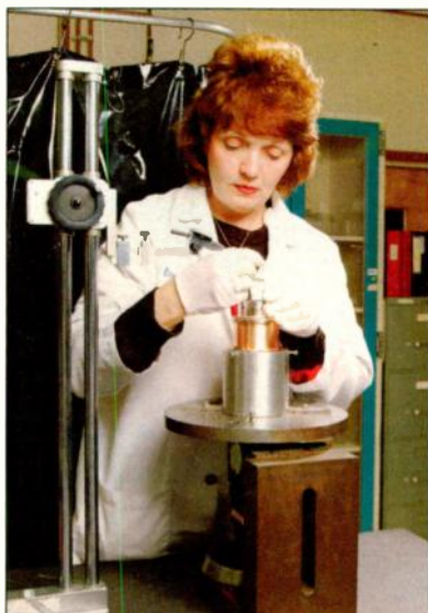
Sandy Kropp performs tests on a small magnetron tube at the L-3 facility.
