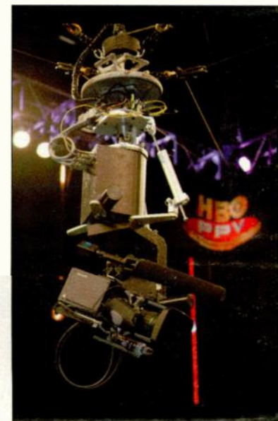
Cablecam's new Nettman Pinpoint Gimbal with the new Panasonic 1500 HD camera and Fujinon 4.7x13 lens, debuted last November on HBO PPV.
