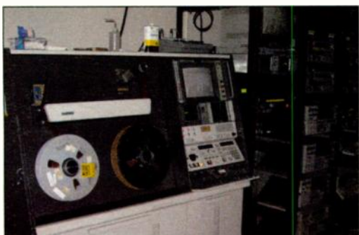
This AVR-3, the last of the quad VTRs produced by Ampex, is needed to play back "Super High Band" recordings at Vidipax.
