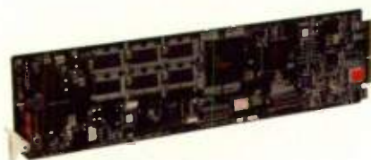
The Cobalt Digital 9821 conversion module
