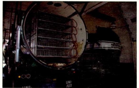
One of the 40-foot long vacuum chambers at Document Reprocessors Middlesex, N.Y. facility, where the Sarnoff Library materials were salvaged.
