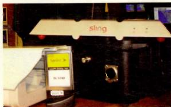
With a Sprint EV-DO card and Slingbox, KPIX has fashioned a remote camera package for $600-$700.
